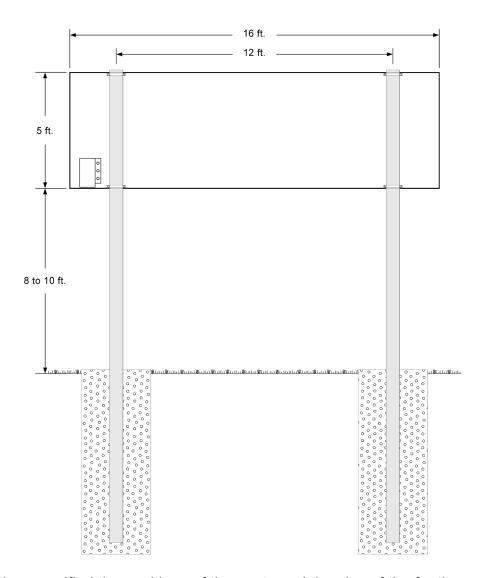
Once you have verified the positions of the posts and the size of the footings, you are ready to dig your holes, pour your concrete, and set your posts. There are several techniques for ensuring proper alignment of the posts. Typically installers will construct a temporary wooden support frame to hold each post in place while the concrete sets. Having plumb posts in the proper position is the key to a smooth mechanical installation.
